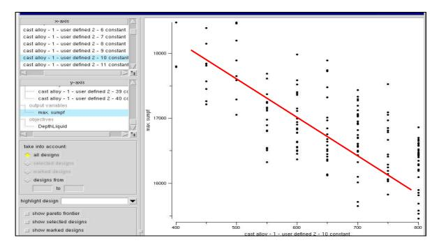
Fig. 4: Scatter chart for a water spray nozzle which belongs to the zone 3. On the x-coordinate the heat transfer coefficient [W/m<sup>2</sup>K] of a spray nozzle is plotted and the y-coordinate shows the liquid pool depth [mm]. A clear tendency can be found.
