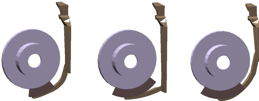
Fig. 10: brake disk with a streamlined gating system, 3 possible layouts
