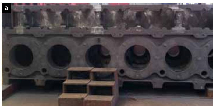
Figure 5: Stress measurements for a 20 ton grey iron casting, with 9 successful measurements (a) and measurements compared to simulation results (b).
