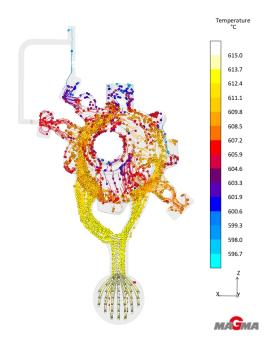
Fig. 2: Visualization of temperatures by virtual particles during the flow in die casting.
