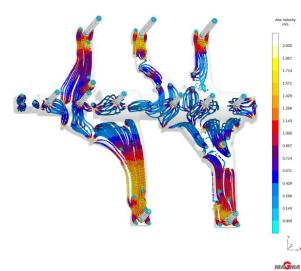
Fig. 3: Representation of air and sand velocities during core shooting using virtual particles.
