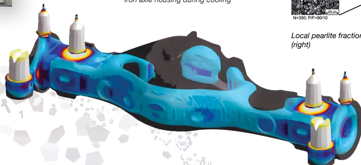
Solidification path for a ductile iron axle housing during cooling
