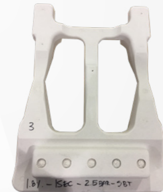
Production core with improved sand compaction and the corresponding sand fraction result after optimizing the tooling
