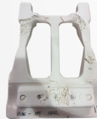
Production core with poor compaction and the corresponding sand fraction result
