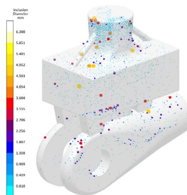
▲ Figure 2: Inclusions diameter tracer result
