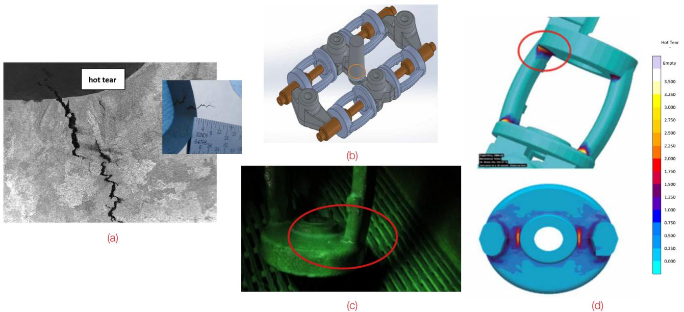
▲ Figure 9: (a) Typical zig-zag fracture pattern of a hot tear; (b) Original situation of the CAD model of the casting; (c) The problem of hot tear defect identified by magnetic particle inspection; (d) Hot tear criterion in simulation showing the critical regions
