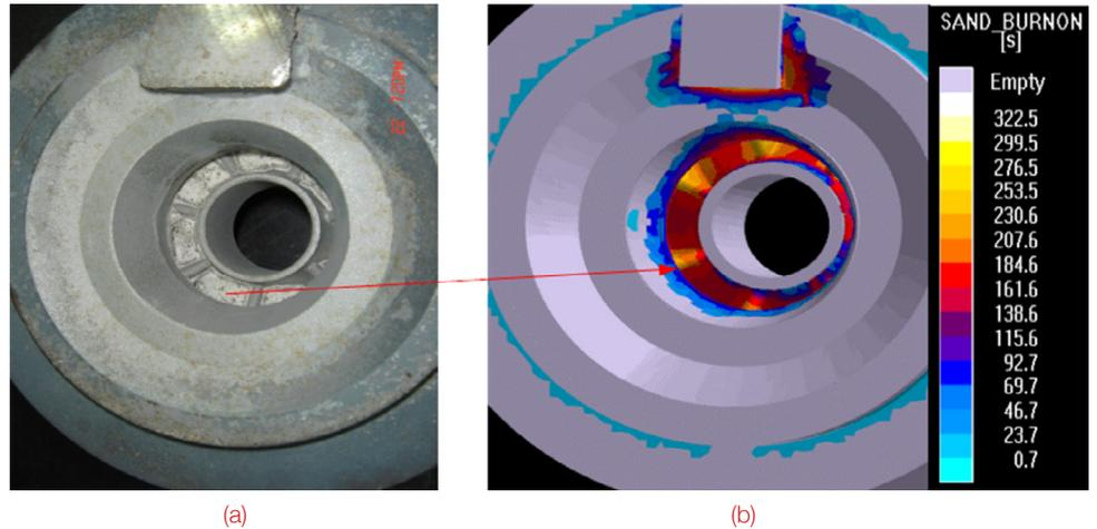
▲ Figure 7: (a) Noticeable burn on defects in center section of casting; (b) Sand burn on simulation results showing the critical regions in the inner center of the casting
