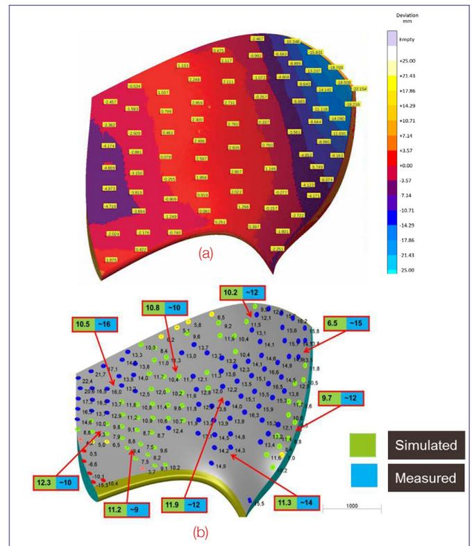
▲ Figure 13: (a) Deviation between the simulated distortion and the target geometry: Initial calculation (b) Deviation between production part and the target geometry. Numbers in green boxes are simulation results and numbers in blue boxes are real measurements (06).
