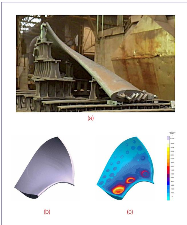
▲ Figure 12: (a) Casting blade of a francis turbine; (b) The geometry of the blade; (c) The liquidus to solidus result from the casting simulation (b) (06)
