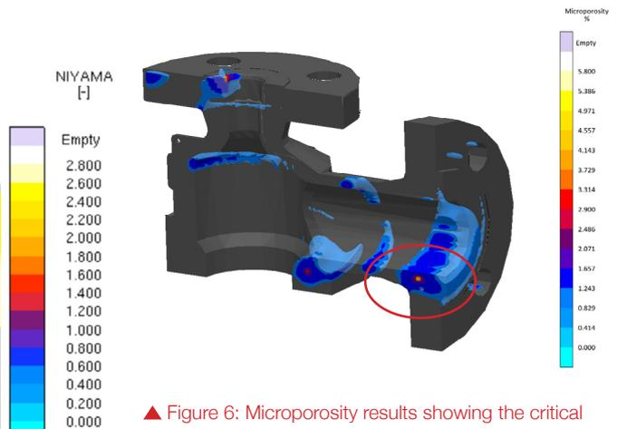
▲ Figure 6: Microporosity results showing the critical region for microshrinkage
