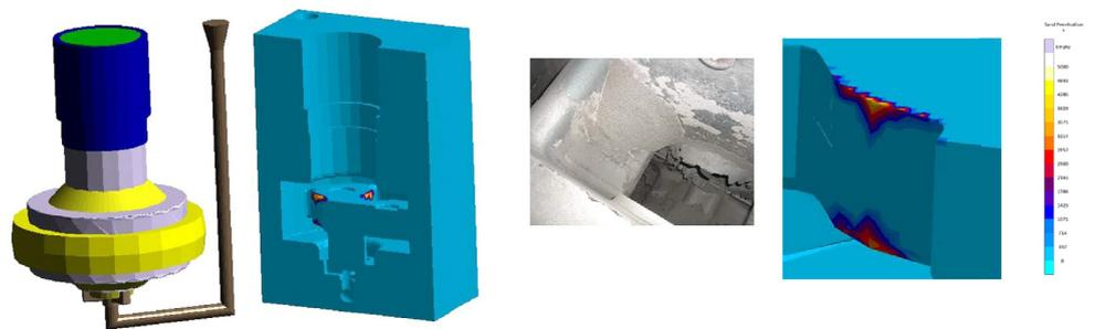
▲ Figure 8: Comparison of predicted and observed penetration defects (03)
