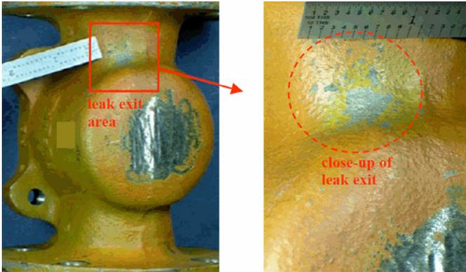
▲ Figure 4: Pump casting investigated to find the root cause of a leak that occurred while in service (02)
