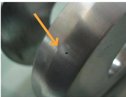
▲ Figure 1: Inclusions in the final casting
