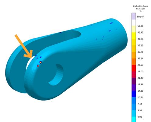
▲ Figure 3: Inclusions area fraction (%), showing in the casting surface the defect of reoxidation inclusion
