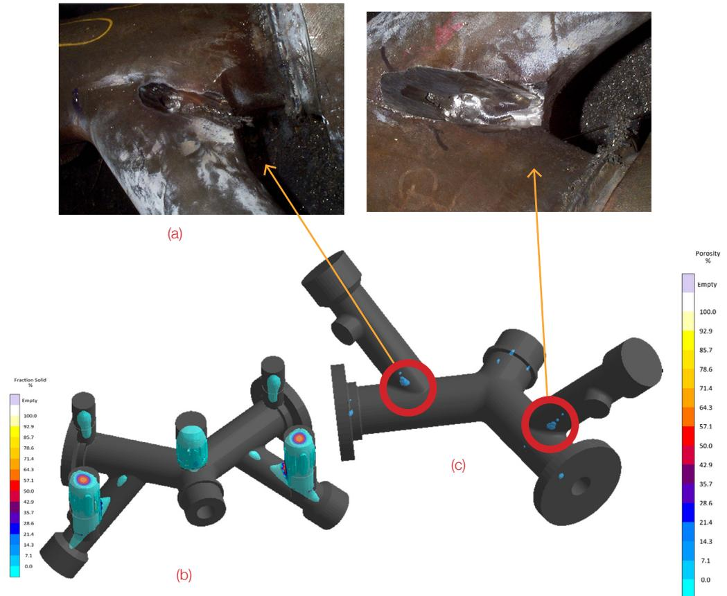
▲ Figure 11: (a) Shrinkage porosity in the practice; (b) Fraction liquid result at the end of solidification, showing regions of liquid isolation; (c) Shrinkage porosity result showing the regions with higher tendency of defect and correlation with the reality
